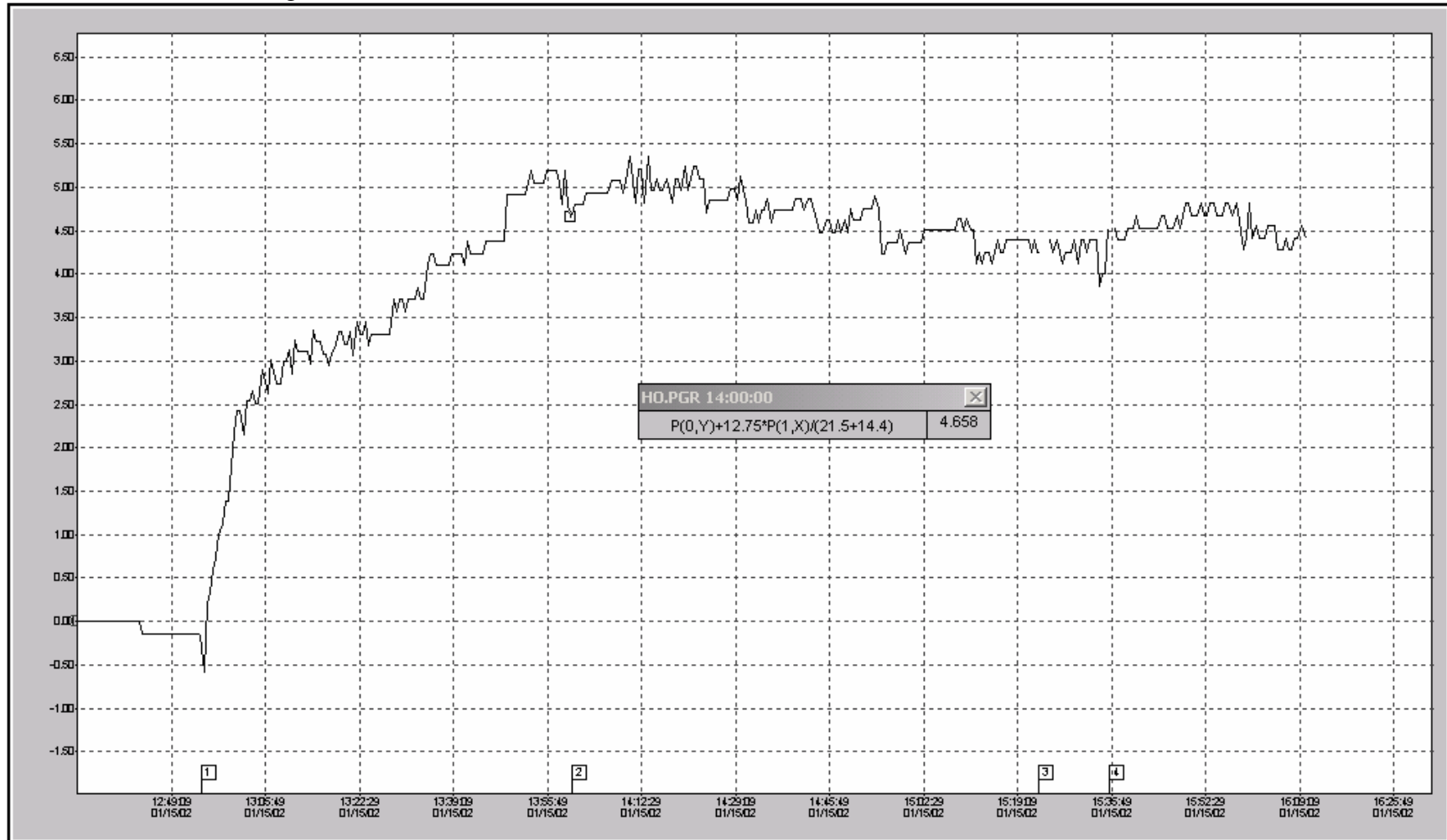
Change in Horizontal Offset when vibration was at its lowest recorded value. +4.658 mils/1”
