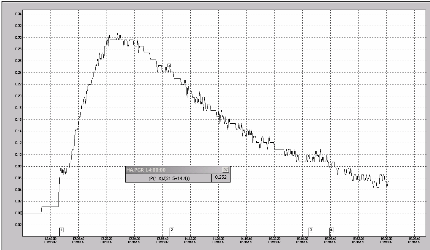
Change in Horizontal Angularity when vibration was at its lowest recorded value. +0.252 mils/1"
